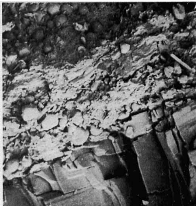
Figure 20—Cross-sectional view of Product S, moistened (about 720X).
